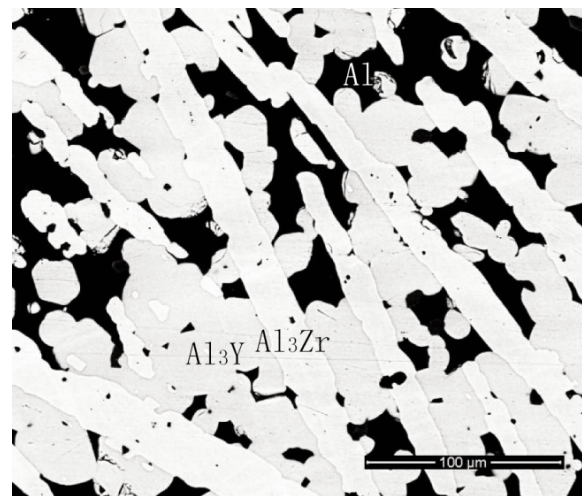
Figure 1. Backscattered electron images of alloy 1# \text{Al}_{78.9}\text{Y}_{12.4}\text{Zr}_{8.8} at 873 K
