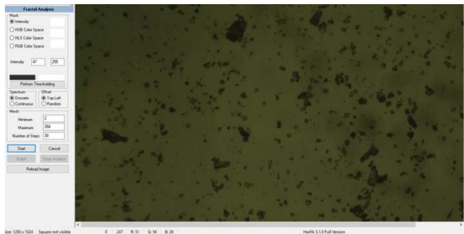
Fig. 8. Image of the sample of the thick flour sample no.1 before thresholding in the software HarFA
