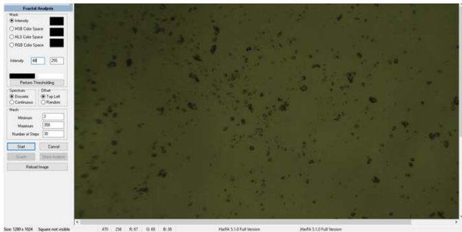
Fig. 2. Image of the sample of the smooth flour sample no. 1 before thresholding in the software HarFA
