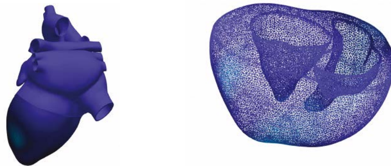
Fig. 12. Large scale model of total heart. a) Displacement simulation b) Mesh generated with 3M finite elements
