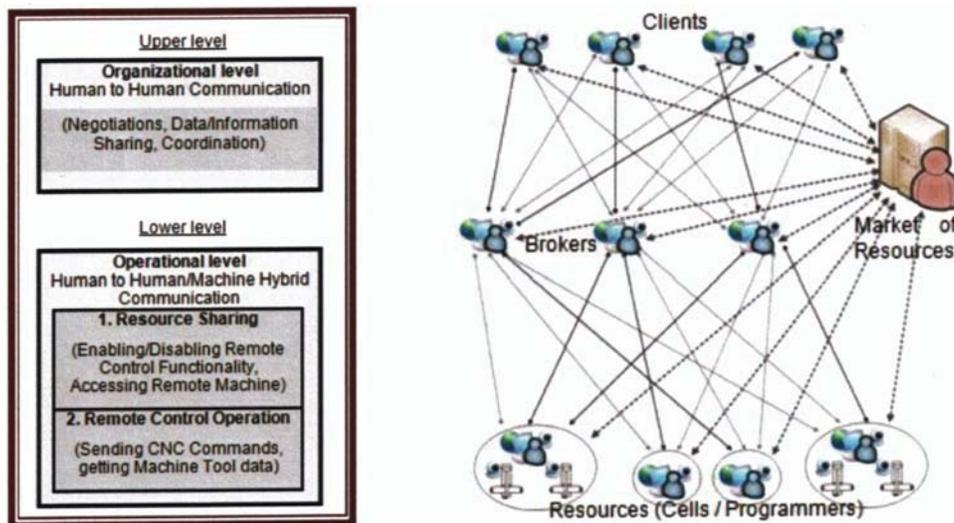
Figure 1. Multiplex communication system levels for remote control and network user communication channels (Putnik et al., 2011 and Shah et al., 2012)
