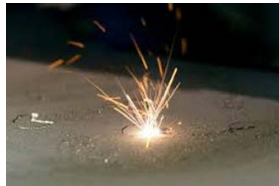
Fig. 9 – Moment of laser melting and sintering the cobalt-chromium alloy.
