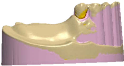
Fig. 4 – Virtual blockout of undercuts (pink color) using available removable partial denture computer-aided design software.
