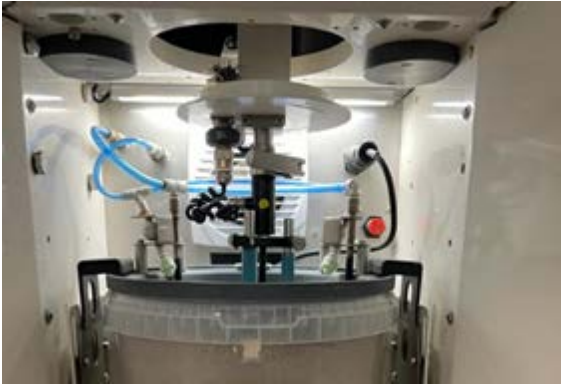
Fig. 10 – Processing of printed metal removable partial denture frameworks by DryLyte technology.
