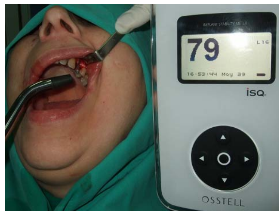
Fig. 2 – Implant stability measurement by means of resonance frequency analysis. The hand-held probe stimulates magnetically the transducer attached to the implant. The degree of implant stability is shown on the display as implant stability quotient value.
