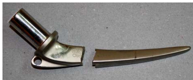
Fig. 9 – Endoprosthesis body fractures due to material fatigue.
