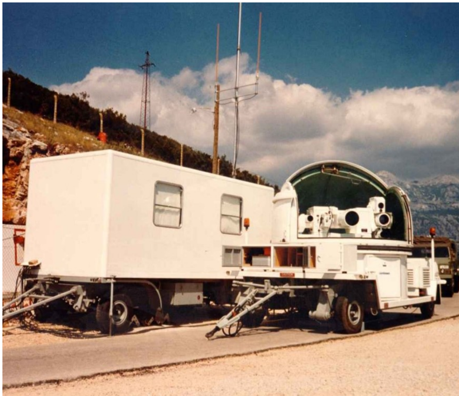
Figure 10 – Optotheodolite system SKYTRACK (Arhiv Vazduhoplovnog opitnog centra, 2016)
