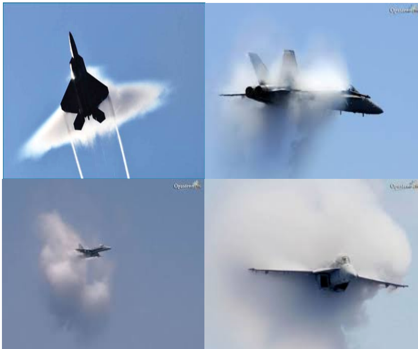
Figure 19 – Display of the visual effects for an aircraft passing Ma = 1 "sound barrier "
