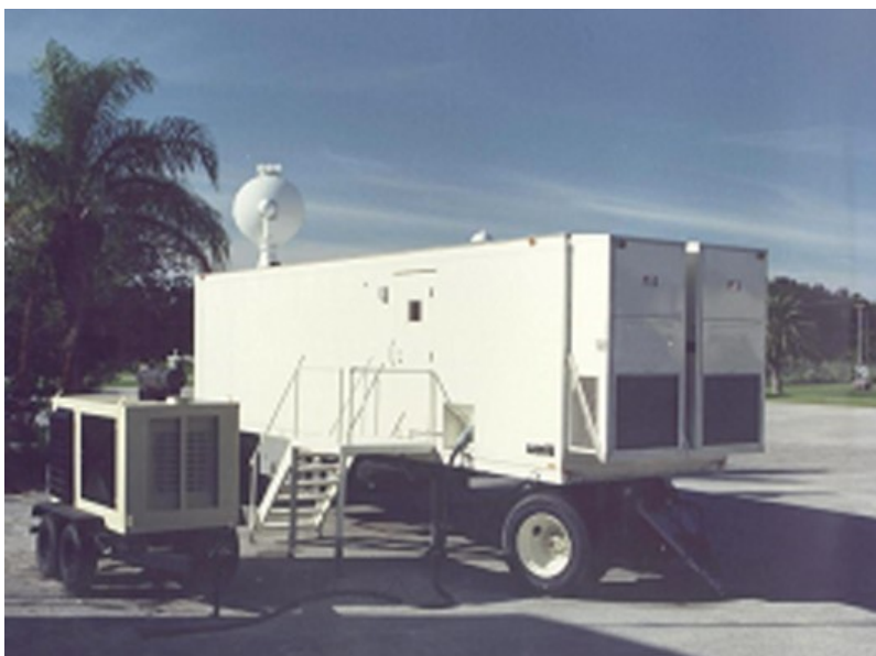
Figure 13 – Telemetry System PCM/FM, US company LORAL - ground receiver mobile station (Arhiv Vazduhoplovnog opitnog centra, 2016)
