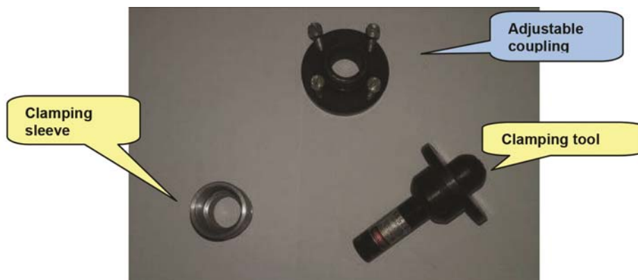
Figure 12 – Parts of the clamping tool for the laser pointer
