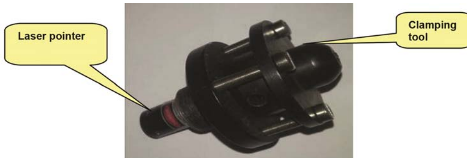
Figure 11 – Clamping tool with a mounted laser pointer
