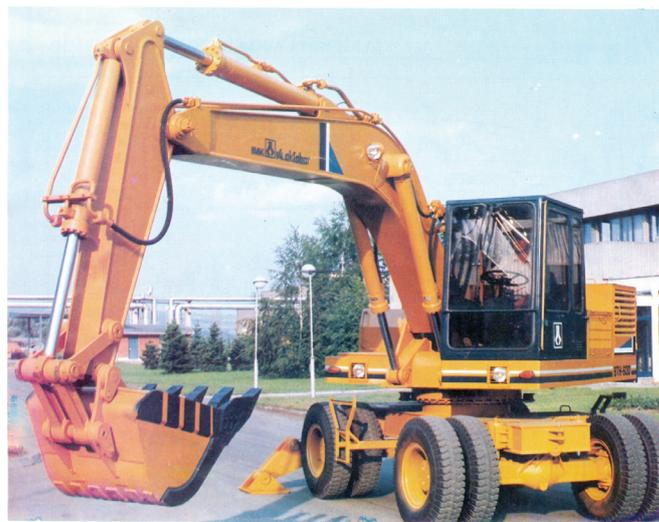
Figure 1 – Physical model of a hydraulic BTH-600 excavator: 1 - undercarriage (pneumatics), 2 - rotary link (platform), 3 - boom, 4 - arm (stick), 5 - bucket
