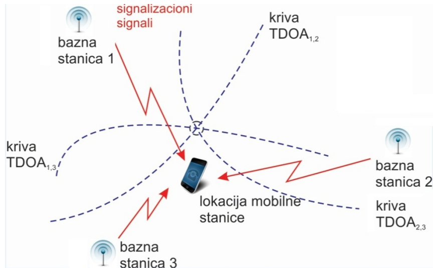
Slika 3 – Određivanje lokacije MS u presečištu tri hiperbole Figure 3 – Determination of the MS location at the intersection of three hyperbolas
