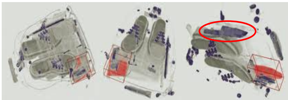
Figure 15 – 3D CT image and the possibility of its rotation in order to find objects that are not visible from the original angle (labeled: ceramic knife and explosive)
