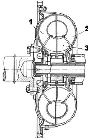
Figure 1 – Scheme of one HDTC
