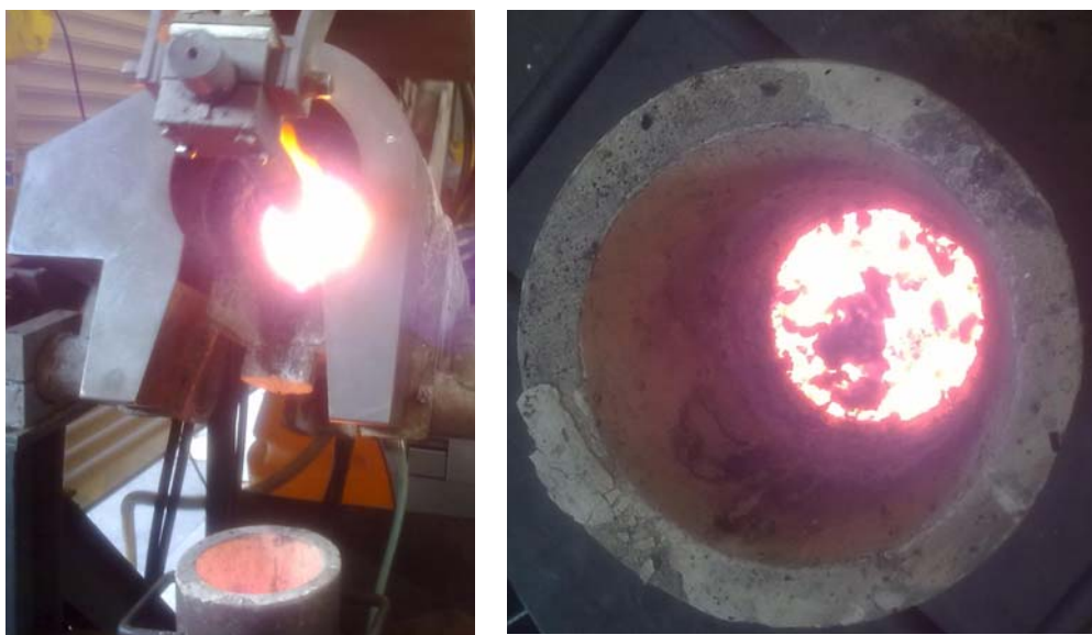
Figure 2 – Reduction smelting of the Rodberg ore in an electric arc furnace (left) and a ladle with the resultant slag (right)
