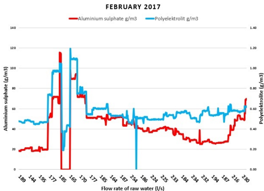
Figure 3a – Dependence of the concentration of added aluminum sulphate and polyelectrolyte on the flow rate of raw water during February 2017
