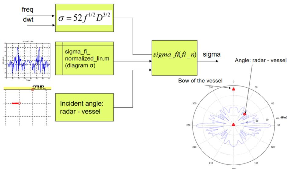
Figure 7 – Model of the radar cross section
