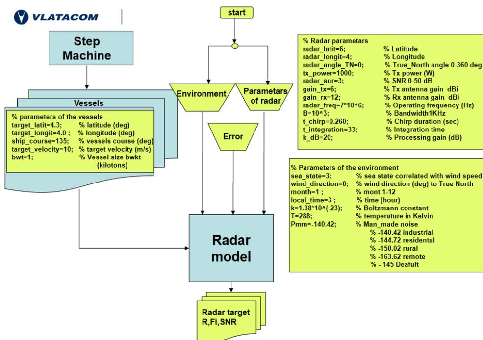
Figure 9 – Flowchart of the OTHR sample simulation
