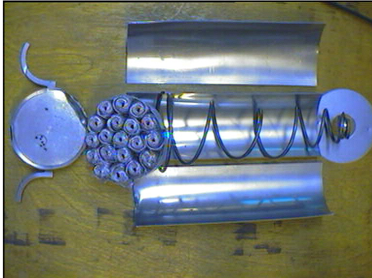
Figure 4 – Parts of an open cluster bomblet with spools and an ejection mechanism (Serbian Armed Forces, 1999)
