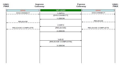
Figure 4 – Termination of a Q-SIG call from Q-SIG, via the SIP, to Q-SIG (Ecma International, 2008)
