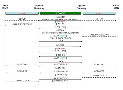
Figure 3 – Establishing a basic Q-SIG call from Q-SIG, via the SIP, to Q-SIG (Ecma International, 2008)
