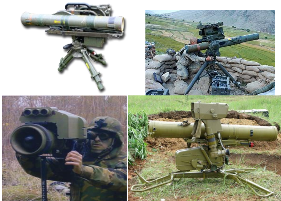
Figure 2 – Second generation ATGMs: MILAN, BGM-71 TOW (upper section); 9K111 „FAGOT“ and „BUMBAR“ (lower section)
