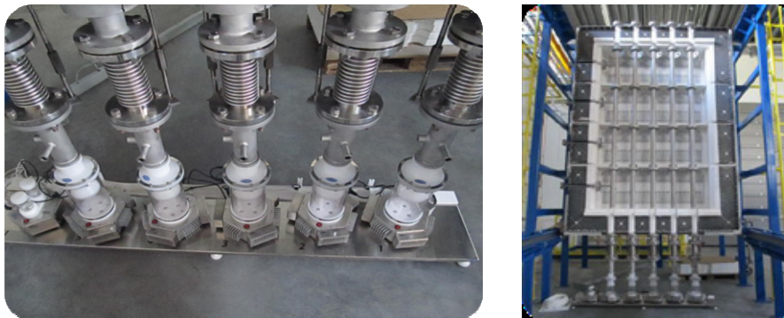
Fig. 9 – USP-generators & wall heated reactors/Scale up of the USP- process (Matula, et al, 2013, pp.1-5)
