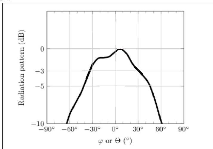
Figure 3 – Example of the radiation pattern of SSB signals (Biscontini, 2021)
