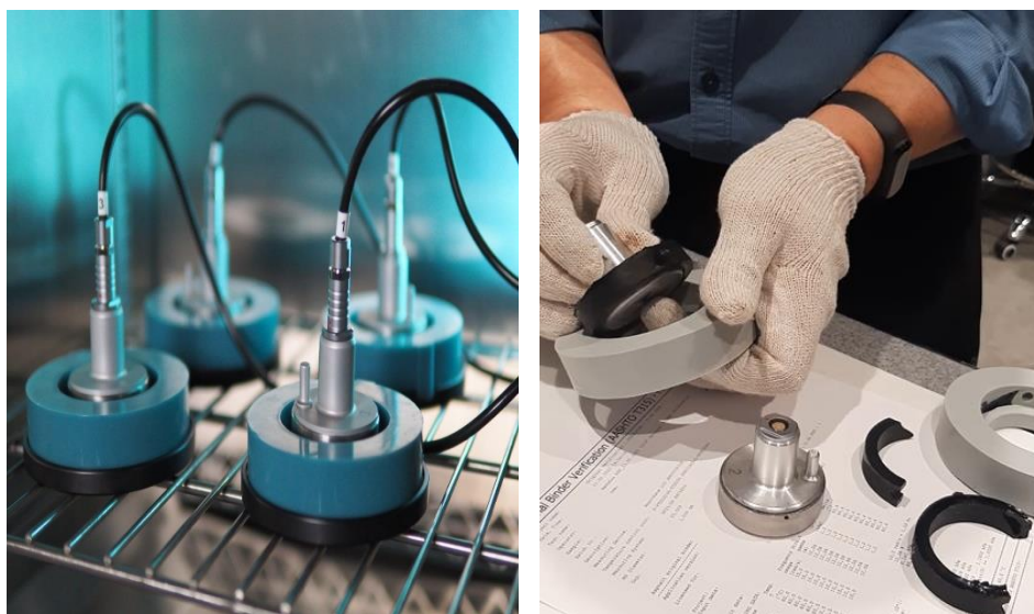
Figure 1 – ABCD sensors during (left) and after (right) testing of binders
