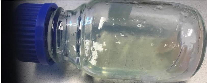
Figure 5 – Formation of silica gel after sulfuric acid leaching at 90°C
