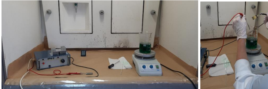
Figure 3 – The laboratory setup for the electrochemical deposition of nickel on brass
