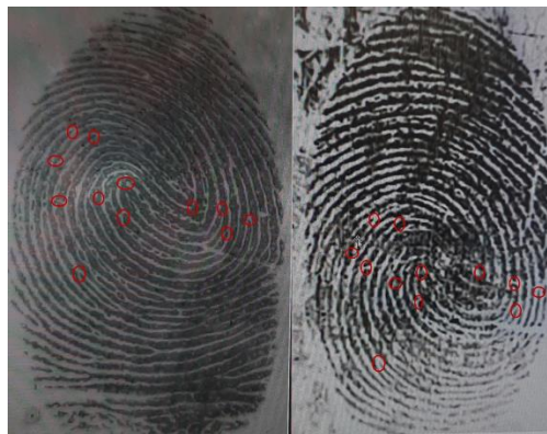
Figure 10 – Development of a fingerprint on the brass surface by the electrodeposition of nickel with the 10 \text{ mA/cm}^2 current density and the 12s deposition time. Some characteristic details of the fingerprints, minutiae (fingerprint developed with conventional magnetic latent print powder Sirchie – left and sample L4 after photo editing - right) are shown
