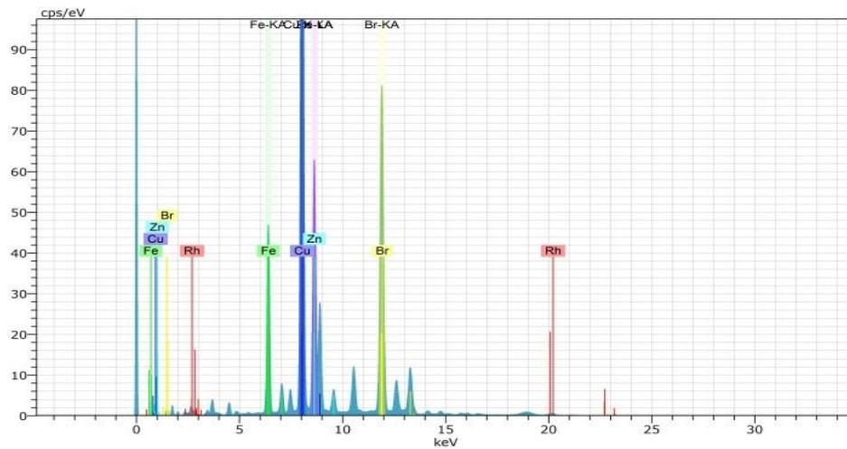
Figure 3 – X-ray fluorescence spectrum of the sample (conductor material)
