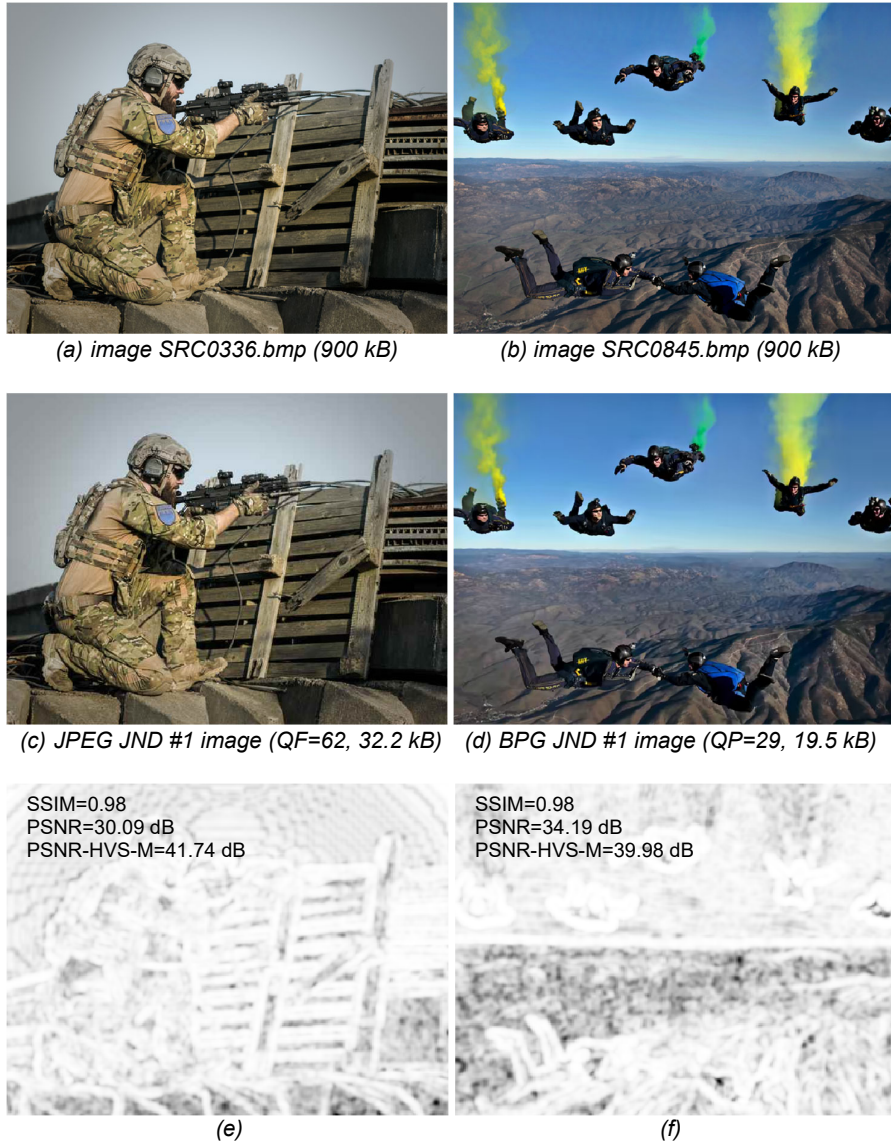
Figure 1 – (a) (b) original images, (c) JPEG JND #1 compressed image, (d) BPG JND #1 compressed image, (e) structural similarity map for JPEG image, and (f) structural similarity map for BPG image
