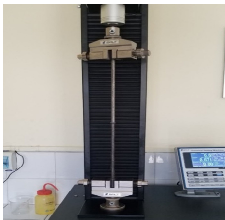
Figure 8 – Deploy an experiment to measure spring hardness
