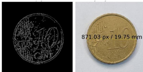
Figure 13 – Coin image processing for pixel-to-millimeter conversion
