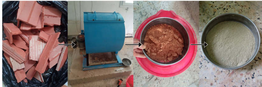
Figure 9 – Crushing presses for brick powder
