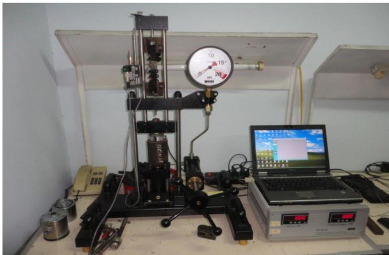
Figure 9 – Force measurement system calibration equipment
