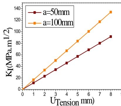
Figure 9 - Effect of Imposed Displacement  $U$  on Mode I Propagation of a Crack ( $U > 0$ , Tension)
