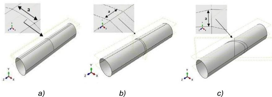
Figure 1 - Pipeline containing a crack: (a) circumferential, (b) longitudinal, (c) mixed (45° orientation)
