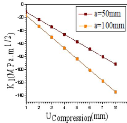
Figure 11 - Effect of Imposed Displacement  $U$  on Mode I Propagation of a Crack ( $U < 0$ , Compression)
