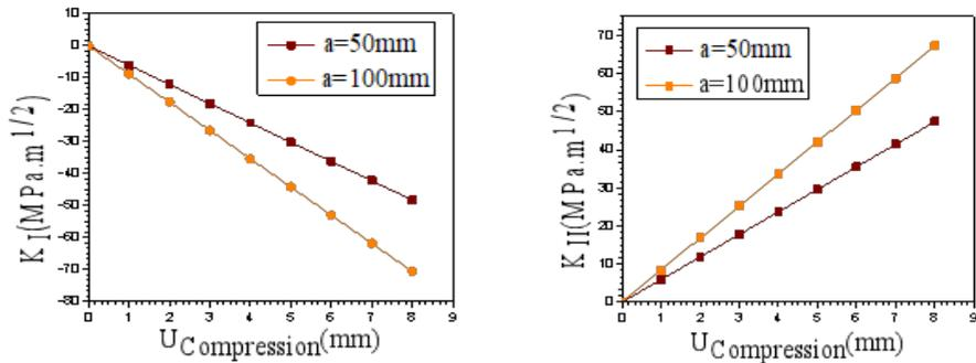
Figure 19 - Effect of Imposed Displacement  $U$  on the Propagation Kinetics in Modes I and II of a Crack Oriented at  $45^\circ$  ( $U < 0$ , compression)
