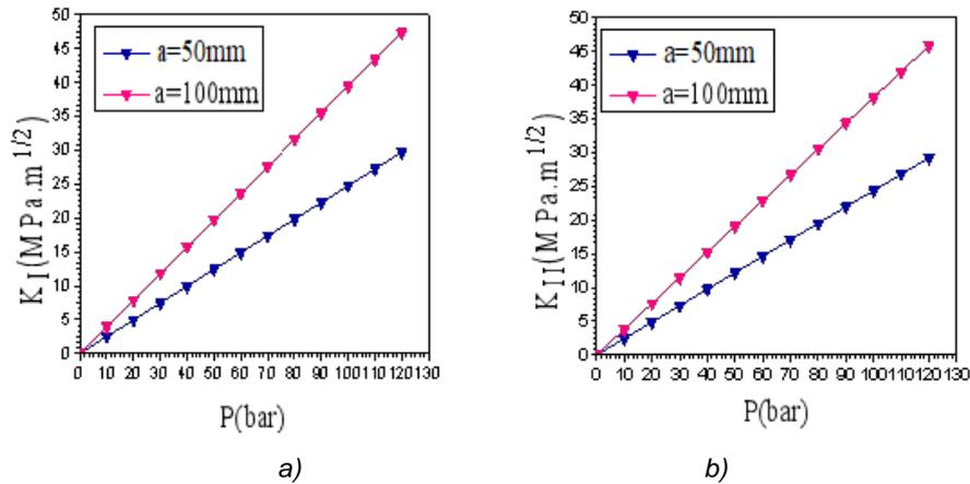
Figure 7- Effect of Internal Pressure on the Mode I and Mode II Behaviour of a Crack Oriented at 45°
