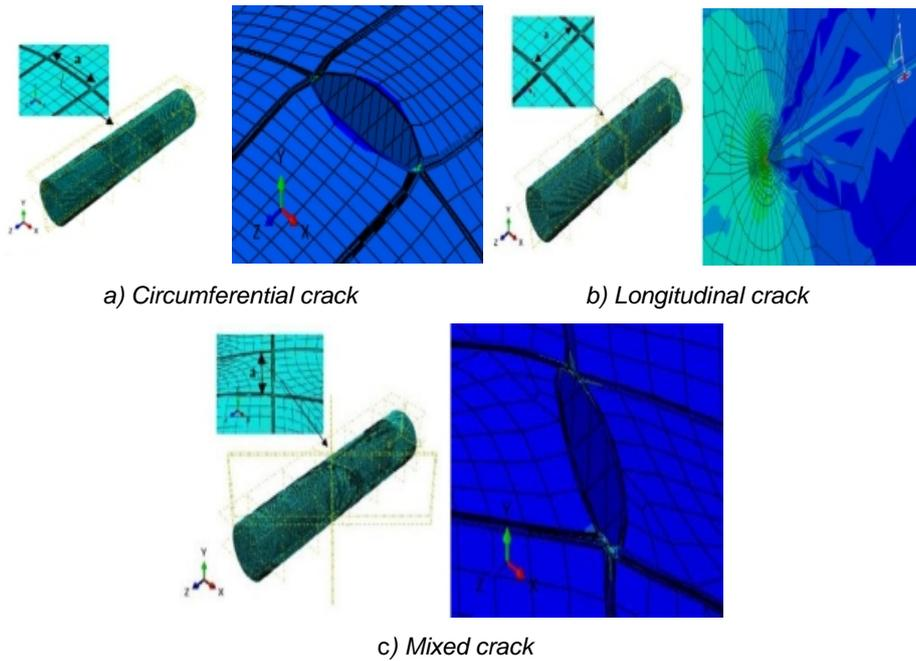
Figure 3 - Mesh of the analysed structure
