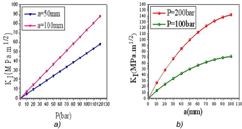
Figure 5 - Effect of Pressure and Longitudinal Crack Size on its Propagation Kinetics in Mode I
