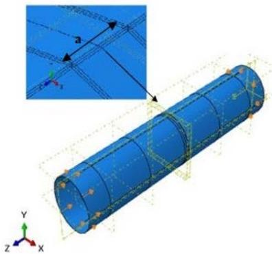
Figure 14 - Boundary conditions for a pipeline with a longitudinal crack subjected to compressive forces
