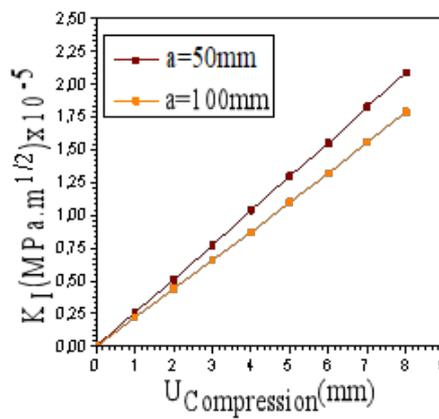
Figure 15 - Effect of Imposed Displacement  $U$  on Mode I Propagation of a Crack ( $U < 0$ , Compression)
