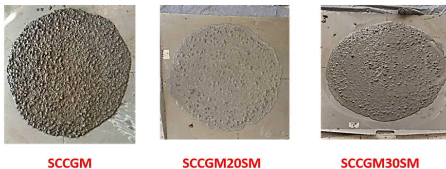
Figure.8 – Visual control of segregation and bleeding of RMA of different SCC mixtures (source author)
