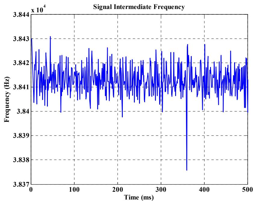
*Figure 4 – Change of the frequency of a typical input signal with the frequency disorder that occurs at one point (at 360ms)*
