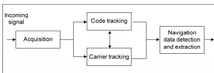
Figure 1 – The block diagram of one GPS receiver channel
