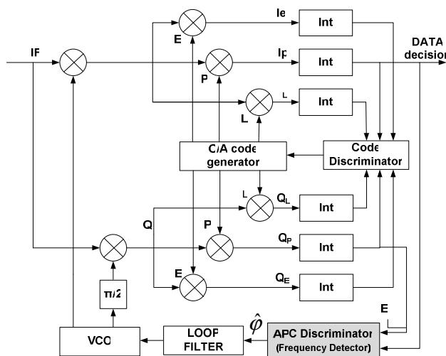
Figure 3 – General configuration used for signal tracking in the GPS software receiver, with the integrated DLL and PLL
