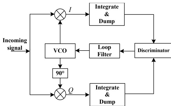
Figure 2 – The block diagram of the Costas PLL
