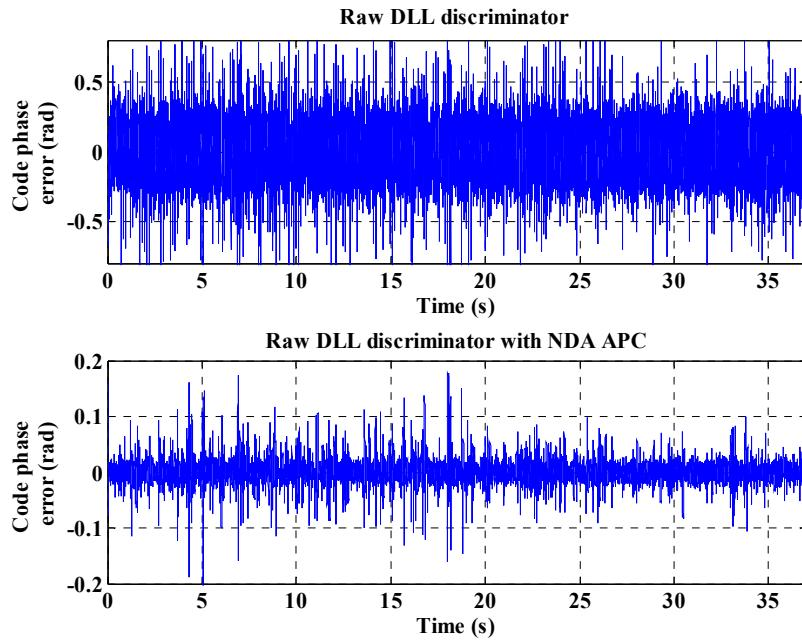
*Figure 7 – Signals at the output of the discriminator (DLL) in the case of the Costas PLL (upper) and the NDA phase estimator (lower)*
