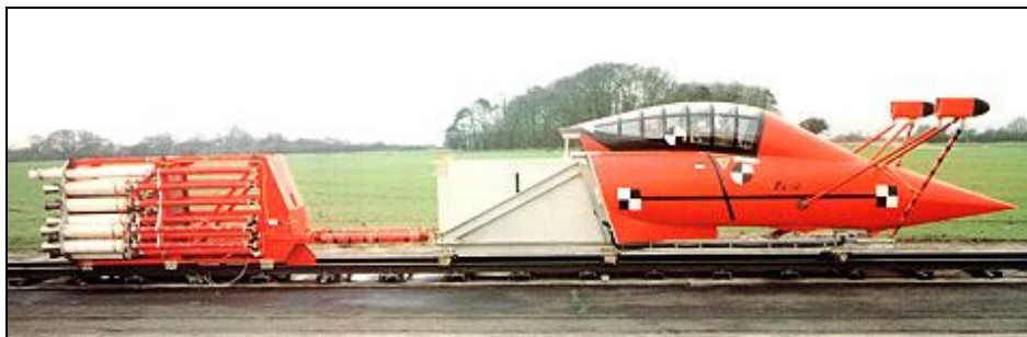
Figure 4 – Martin Baker Eurofighter rocket sled
