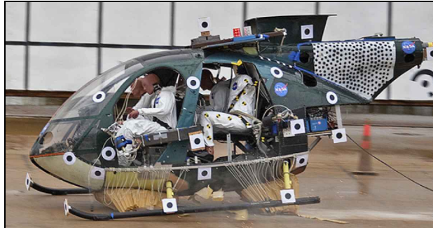
Figure 9 – Crash-test of a helicopter MD-500 with a crew of four anthropometric dummies - Hybrid III dummies
