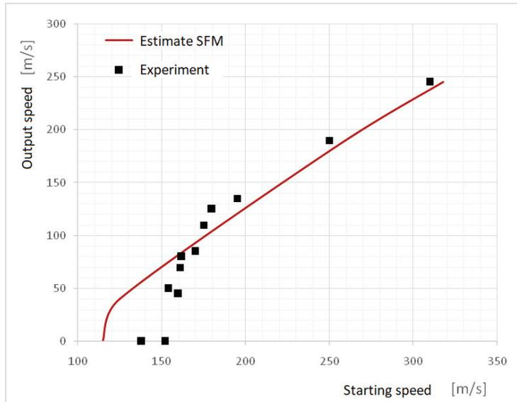
Figure 7 – Analysis of the SFM by a blunt projectile for a plate with a thickness of 8 mm
