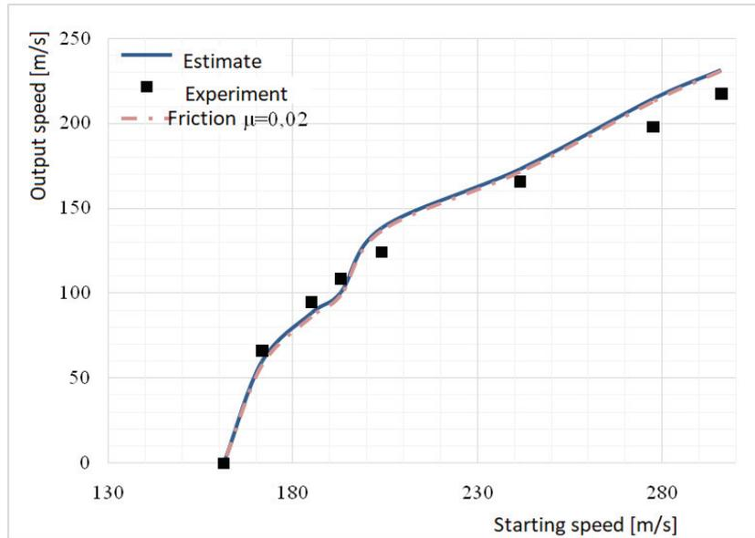
Figure 14 – FEM analysis by a blunt projectile for a plate of 10 mm thickness
