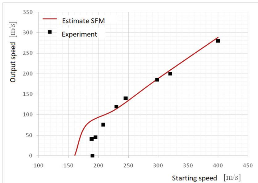
Figure 9 – Analysis of the SFM by a blunt projectile for a plate with a thickness of 12 mm
