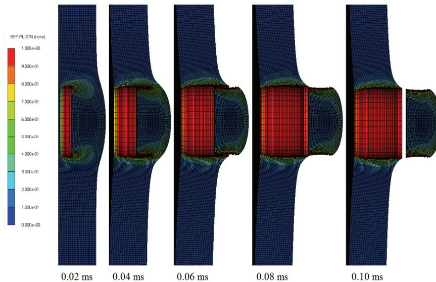
Figure 18 – Perforation of a steel plate with a blunt projectile (FEM method)
