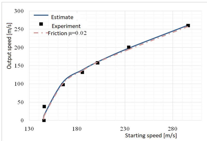
Figure 12 – FEM analysis by a blunt projectile for a plate of 6 mm thickness
