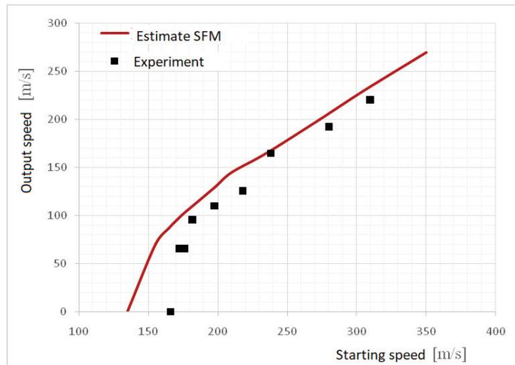
Figure 8 – Analysis of the SFM by a blunt projectile for a plate with a thickness of 10 mm
