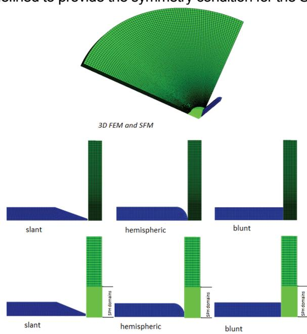
Figure 3 – 3D and 2D FEM and SFM projector networks and projectiles
