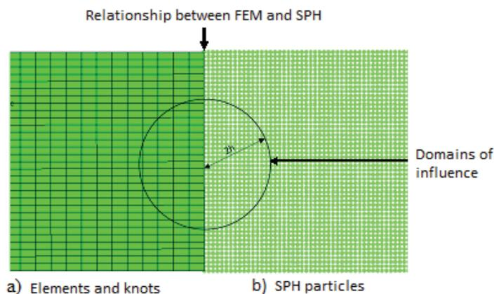
Figure 2 – Coupled SPH and FEM methods
