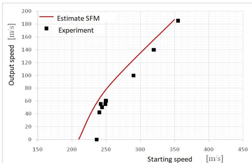
Figure 10 – Analysis of the SFM by a blunt projectile for a plate with a thickness of 16 mm
