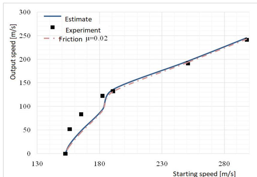
Figure 13 – FEM analysis by a blunt projectile for a plate of 8 mm thickness
