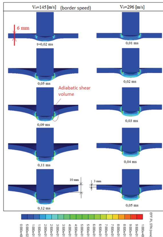
Figure 35 – Comparison of blunt projectile penetration through a 6mm-thick steel plate at two speeds,  $V_0=145$  m/s and  $V_0=296$  m/s, FEM method
