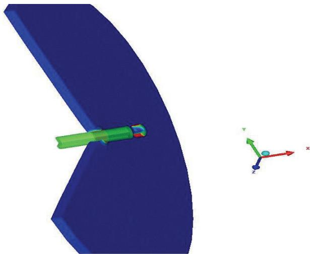
Figure 19 – 3D Flat Perforation of a steel shell with a blunt projectile (FEM Method)
