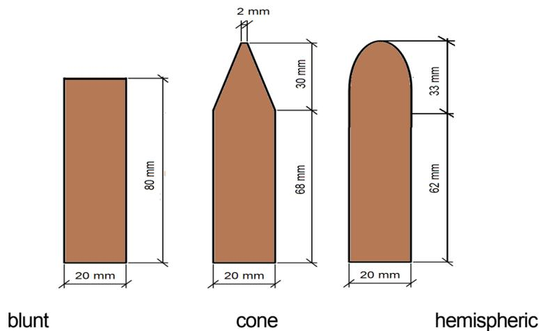
Figure 1 – Geometry and dimensions of projectiles with different tip shapes
