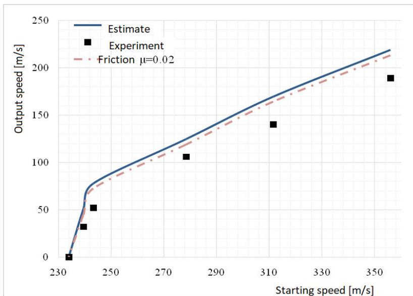
Figure 16 – FEM analysis by a blunt projectile for a plate of 16 mm thickness
