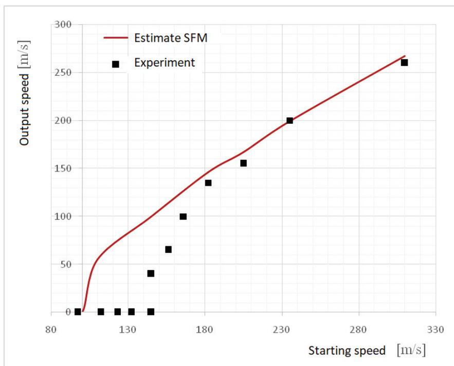
*Figure 6 – Analysis of the SFM by a blunt projectile for a plate with a thickness of 6mm
