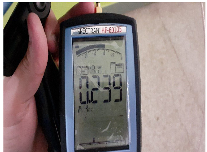
Picture 3b. Example of measuring the electric field strength using the instrument Spectran HF 60105
