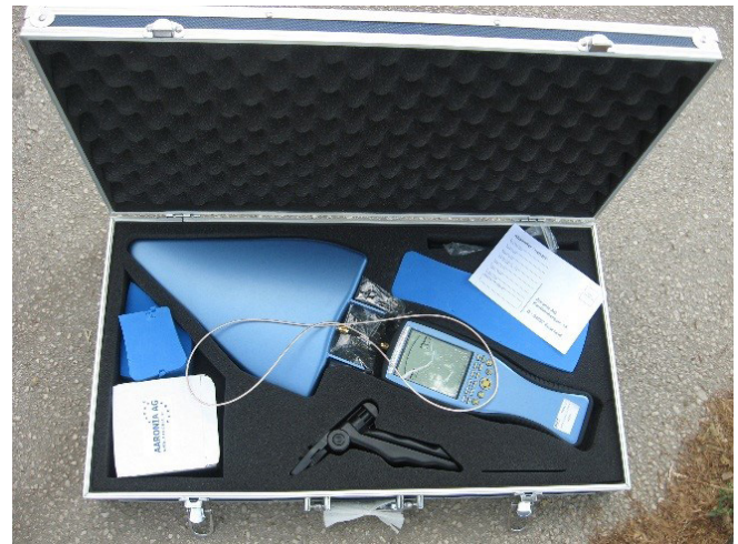
Picture 1. Instrument Spectran HF 60105 for measuring the parameters of high frequency electromagnetic radiation
