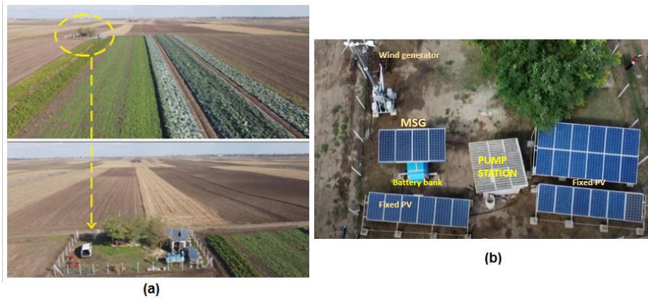
Figure 3. The drone shoot of the "Smart Land" and hybrid power for irrigation and remote management on the plot "Belegiš"; (a) view of the plot (above) and view of the hybrid power plant based on RES (below), (b) disposition of hybrid power
